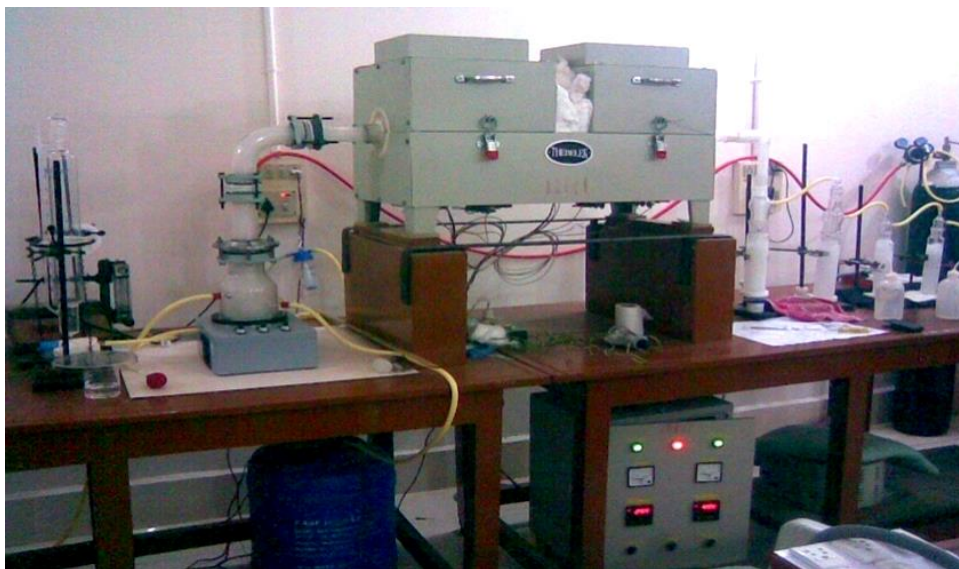
Figure 1. Photograph of ultrasonic atomization and pyrolysis technique.
